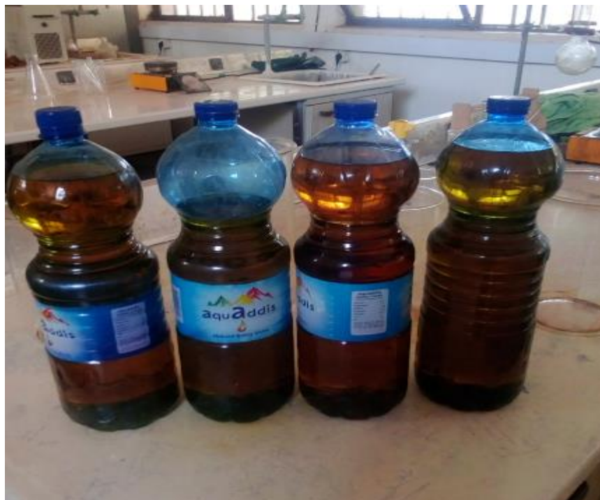
Figure 3.8. The final collected pure biodiesel
