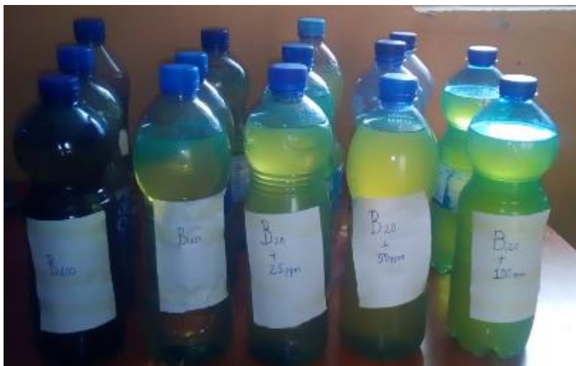
Figure 3.13. Biodiesel and diesel-biodiesel blend ready for characterization
