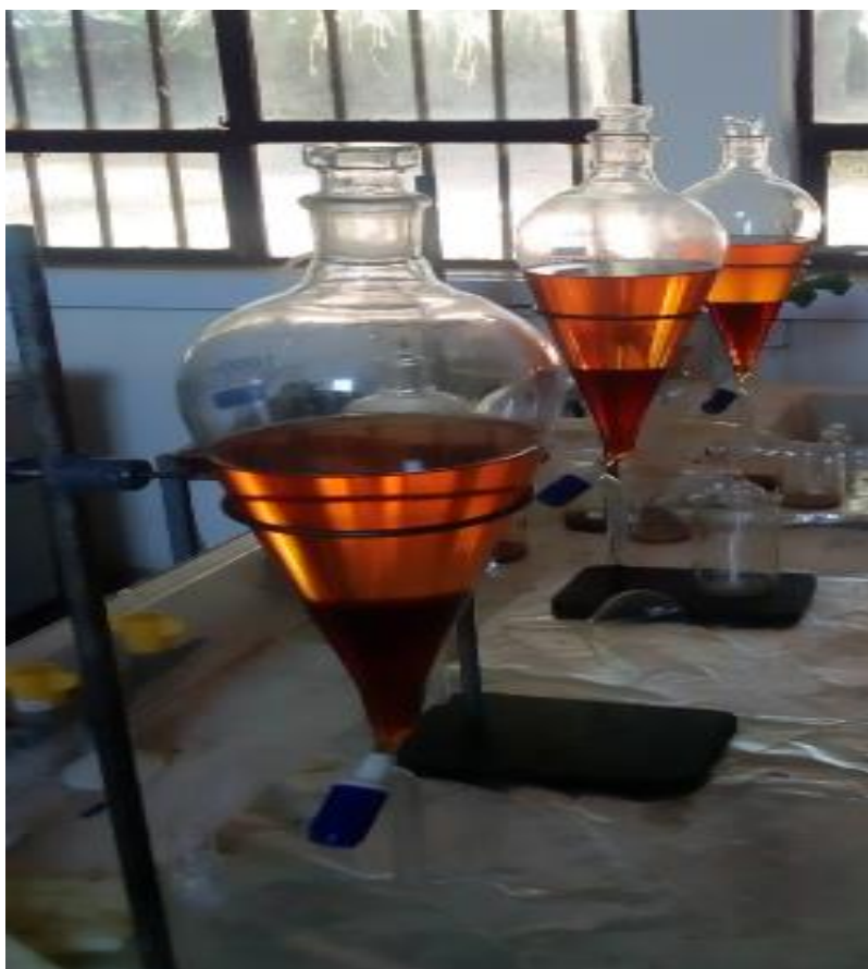
Figure 3.5. Separation of biodiesel and glycerol
