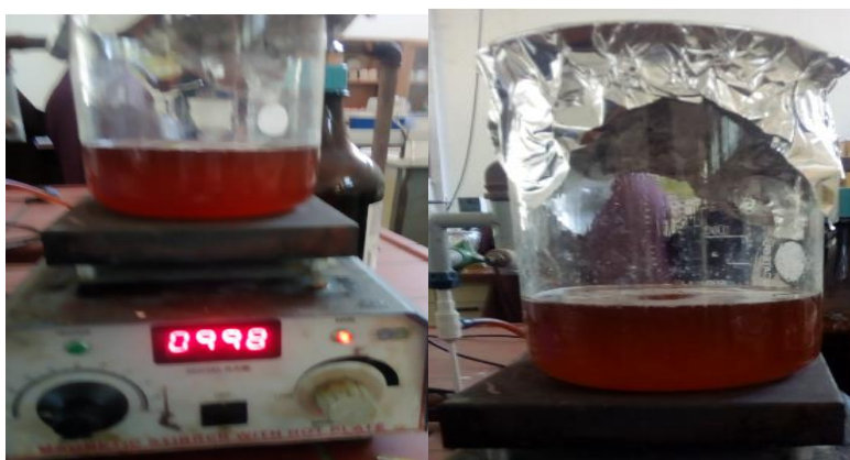
Figure 3.4. Heating the mixtures of KOH and methanol with oil
