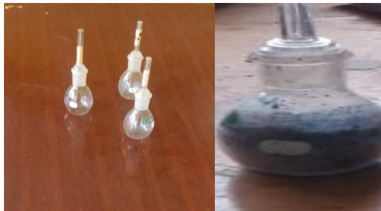
Figure 7. Specific gravity test in the laboratory (Source: photos taken during Specific gravity test)
