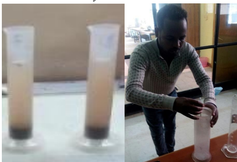
Figure 10. Free swell test laboratory (Source: photos taken during test)
