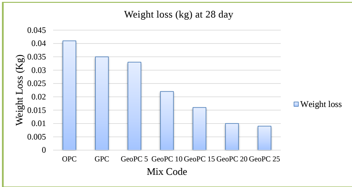
Figure 4. 10 Sulfate attack of Concrete at 28 Days of Curing
