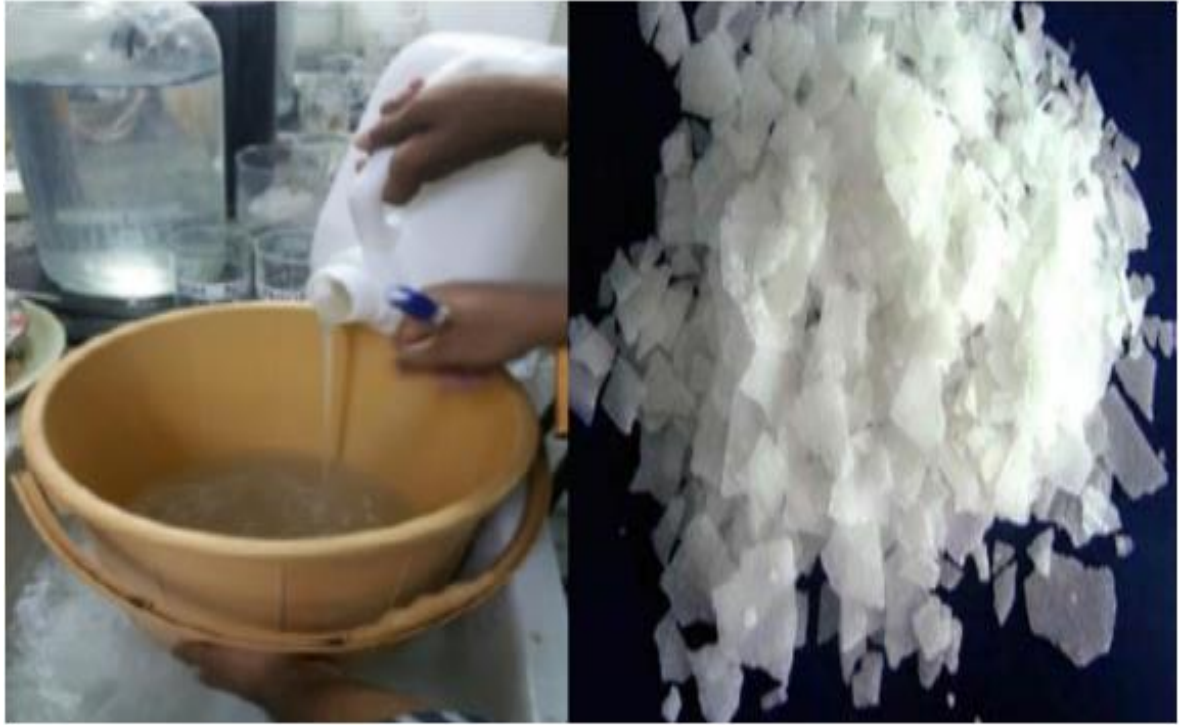
Figure 2. 2 Sodium silicate and Sodium hydroxide pellets (alkaline activators)
