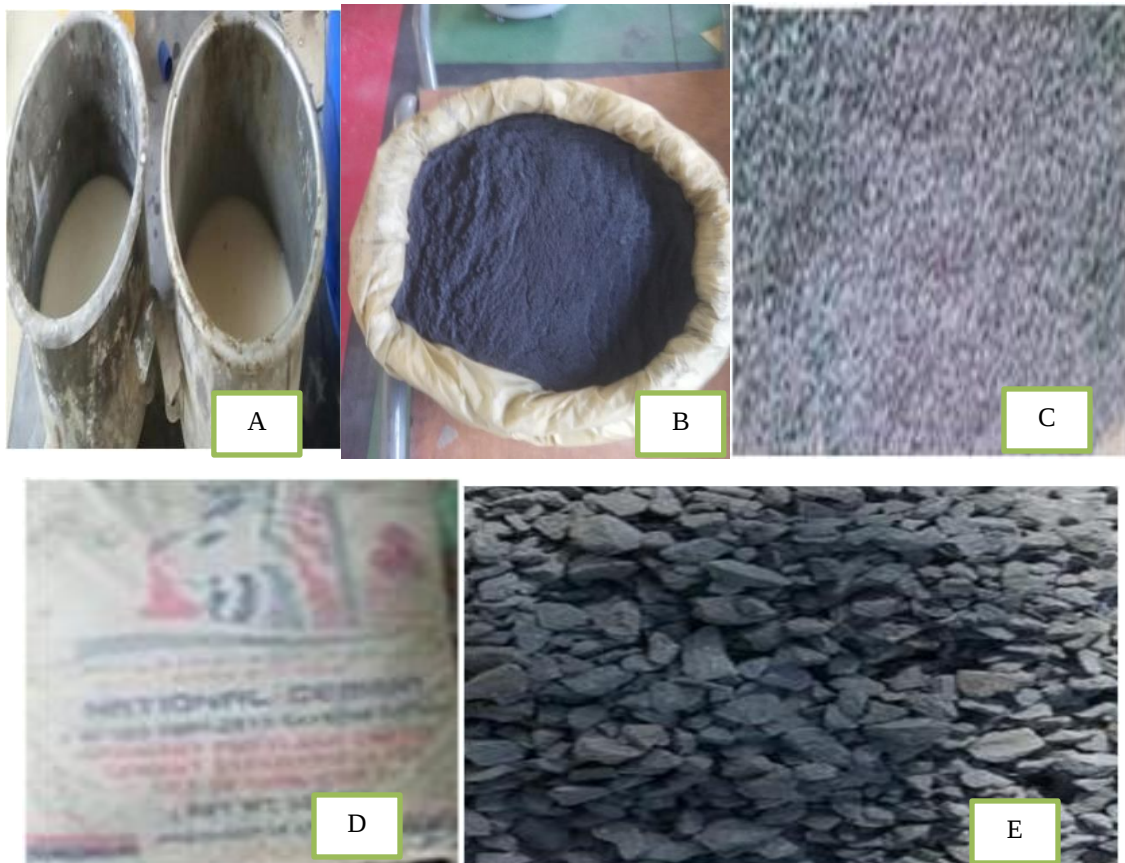
Figure 3. 1 Materials used; A) Alkaline Activator B) SCBA, C) Fine Aggregate, D) National OPC cement, and E) Coarse Aggregate
