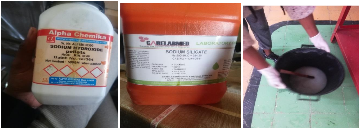
Appendix D 2 : Picture taken during Preparation of Alkaline Activator Solution
