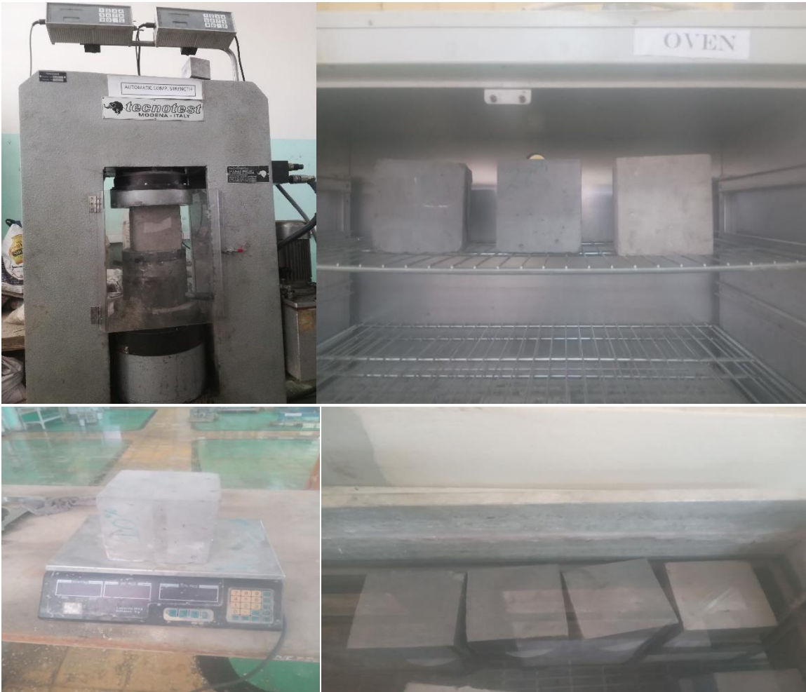
Appendix D5: Pictures shows tests for compressive, water absorption test and Sulfate attack.
