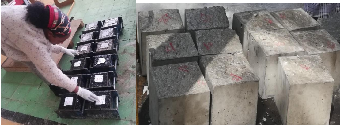
Appendix D4: Pictures shows casted samples: (150*150*150) mm sized cube for compressive, water absorption test and Sulfate attack test.
