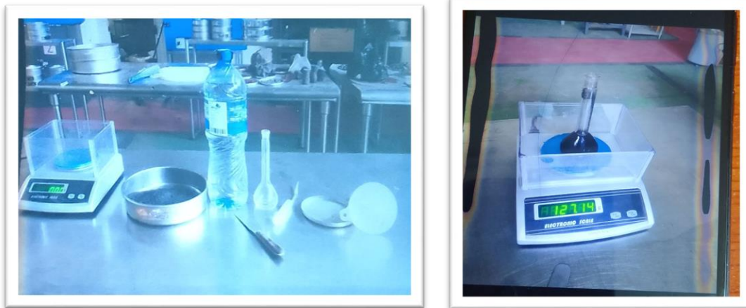
Figure 3. 6 Apparatus and kerosene used to conduct specific gravity of the SCBA. From obtained data, the specific gravity of CBSA was calculated through equation 3.11.
