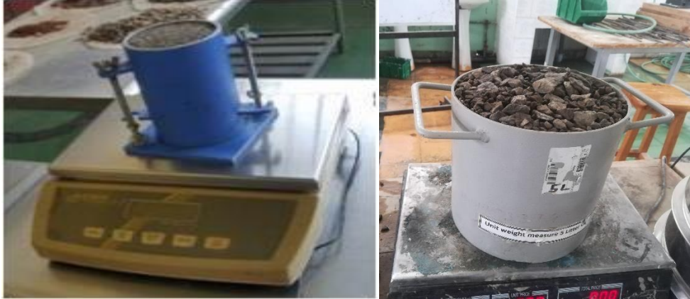
Appendix D 1 : Pictures captured during conducting unit weight test for fine aggregate and Coarse aggregate.
