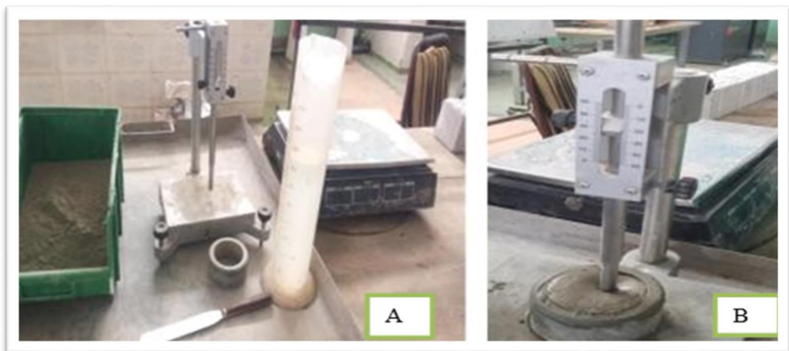
Figure 3. 7 Vicat Apparatus (A), Normal Consistency Test (B)
