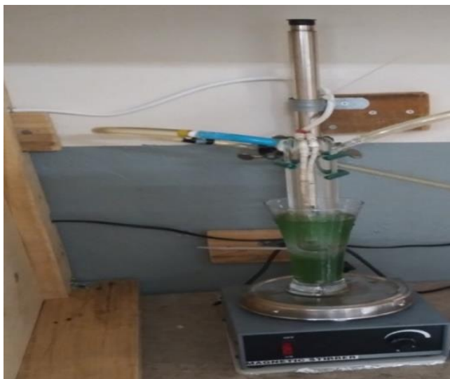
Figure 3. 4: Setup for photocatalytic experiments.
