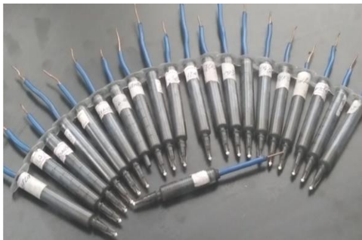
Figure 3.5: Fabricated working electrodes using \text{Ni}_{0.75}\text{Zn}_{0.25}\text{RE}_x\text{Fe}_{2-x}\text{O}_4 and \text{Ni}_{0.75}\text{Zn}_{0.25}\text{RE}_x\text{Fe}_{2-x}\text{O}_4@\text{rGO} .
