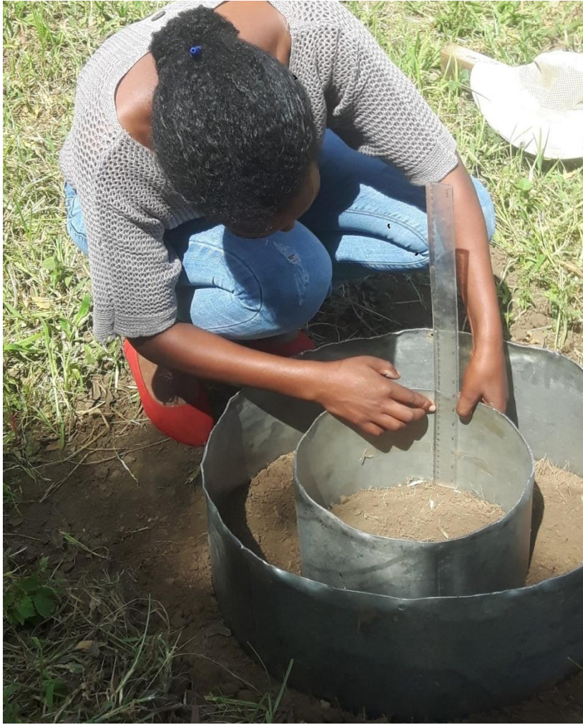
Figure 3 Installation of double infiltrometer for infiltration measurement
