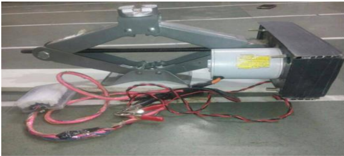
Figure 2. 6: Side view of the modified electric jack (B. Babu, et al. , 2017)
