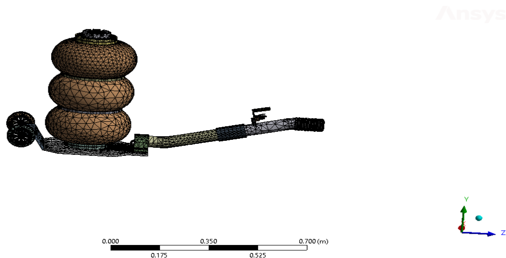
Figure 3. 10: Meshed model of extended handle pneumatic bag floor jack
