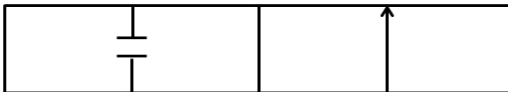
Figure 2. 4: Symbol of a 2/2 directional control valve (Bobbili Seshagiri Rao, 2017)
