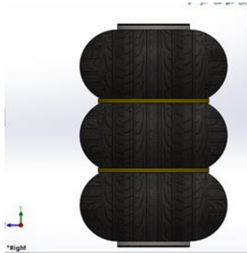
Figure 3. 4: Pneumatic air bag jack assembly
