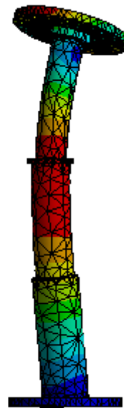
Figure 4. 17: Total deformation of the telescopic shaft at frequency 659.2 Hz
