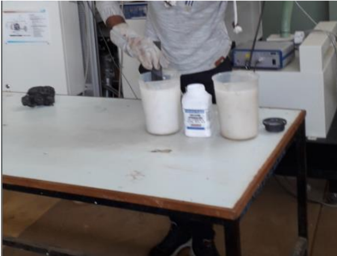
Figure 3.4 Mixing calcium hydroxide with pure water
