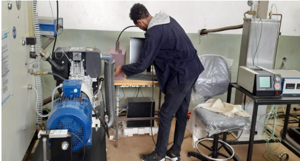
Figure 3.7 Start test by inserting exhaust gas analyzer sensor in HAS
