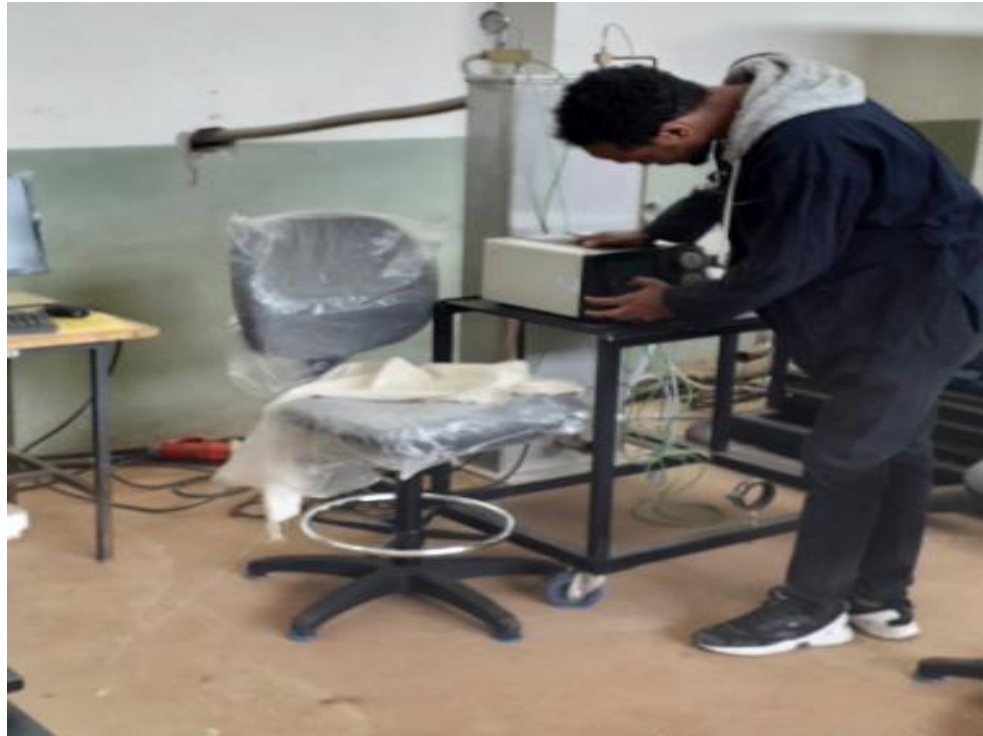
Figure 3.6 Check up and adjust the exhaust gas analyzer before test start
