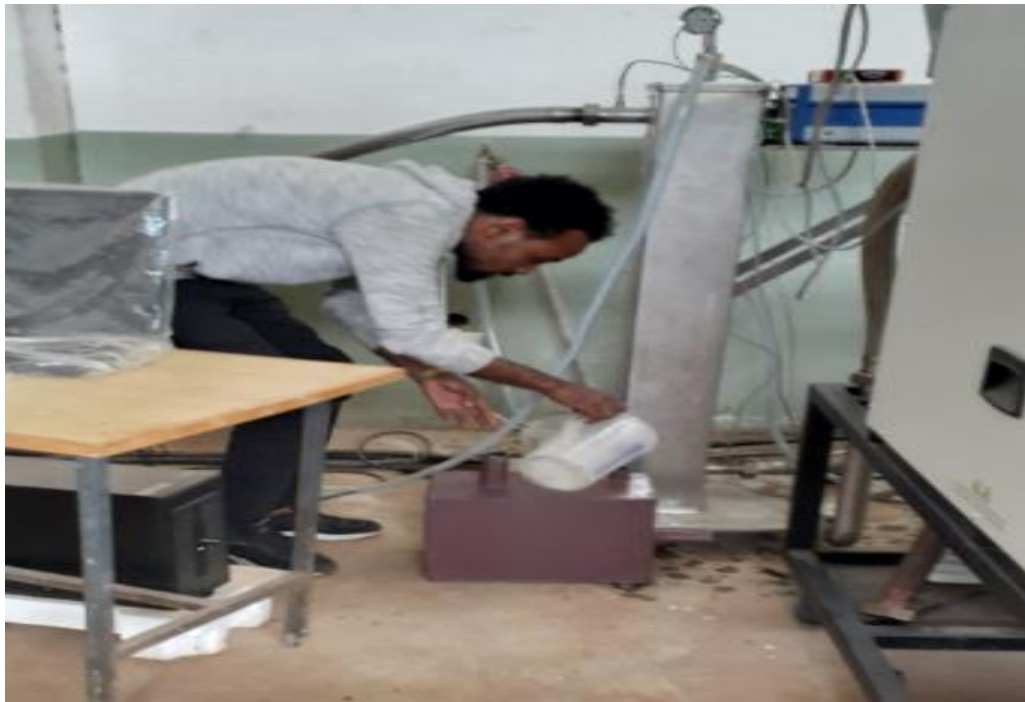
Figure 3.5 Adding lime water to the tank.
