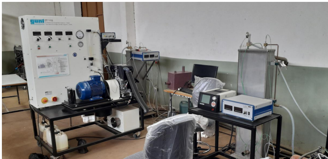
Figure 3.8 a) Single cylinder diesel engine setup and
