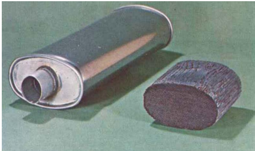
Figure 2.6 Catalytic converter components (John matthey, 2009)
