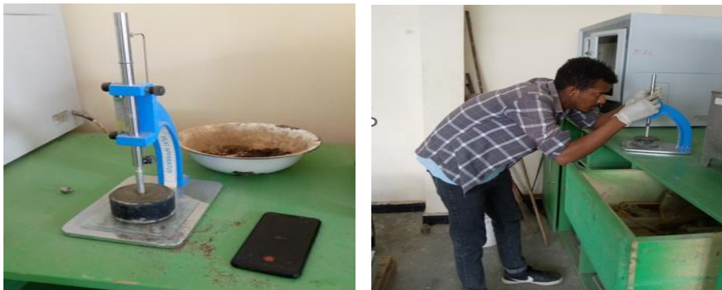
Figure 3-8 Normal consistency and Setting time test by using Vicat apparatus
