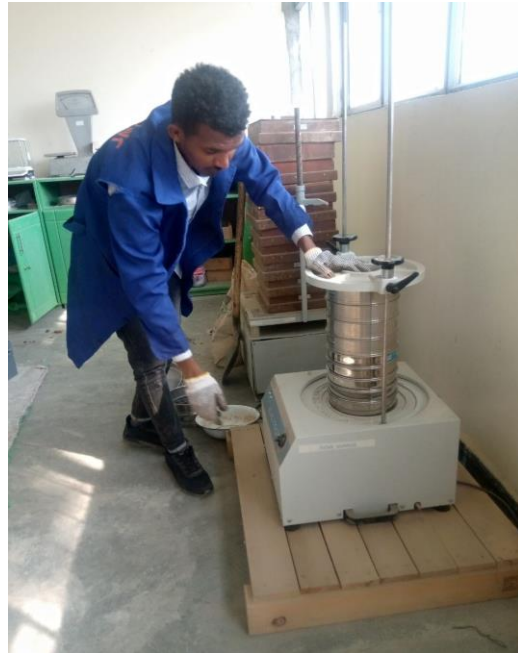
Fine and Coarse Aggregate sieve Analysis
