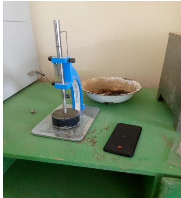
Cement Consistency and Setting Time Test
