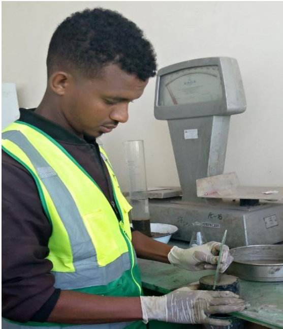
Cement Consistency and Setting Time Test
