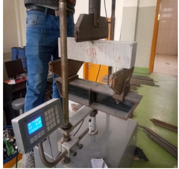
Beam under flexural testing Machine
