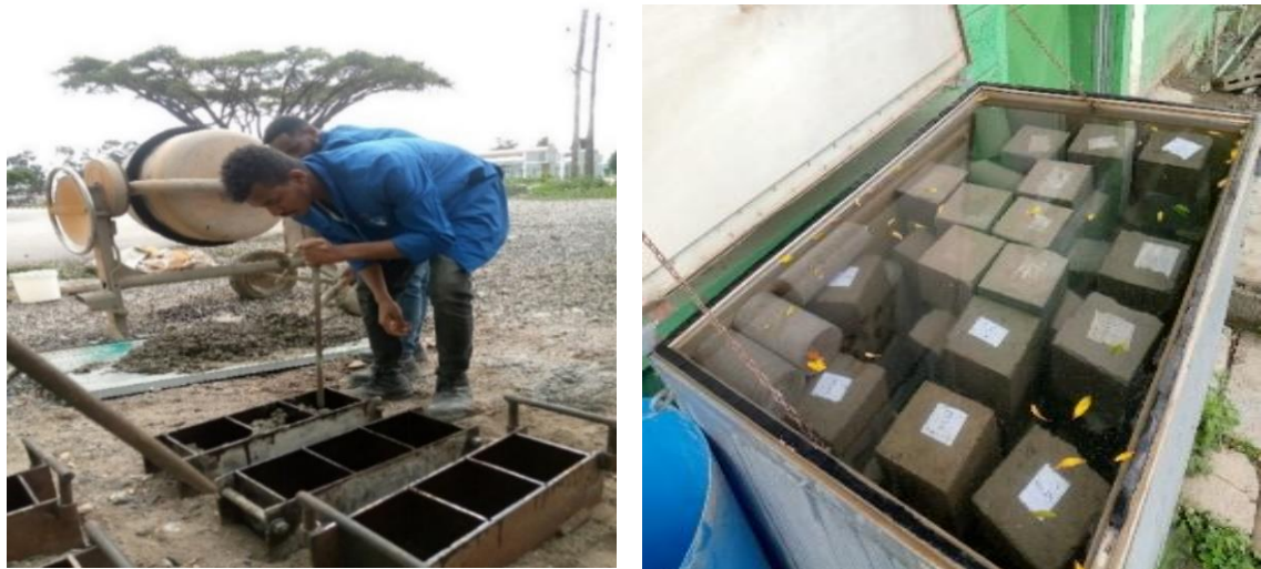
Figure 3-15 concrete sample preparation and curing
