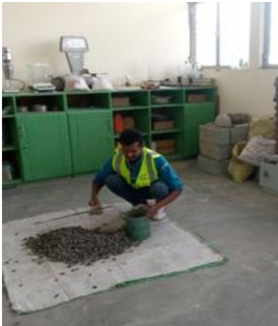
Unit weight and water absorption of Coarse Aggregate
