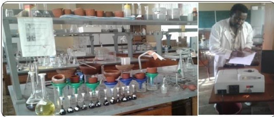
Figure 38. Preparation of the standard solution of nitrite before UV-detections.
