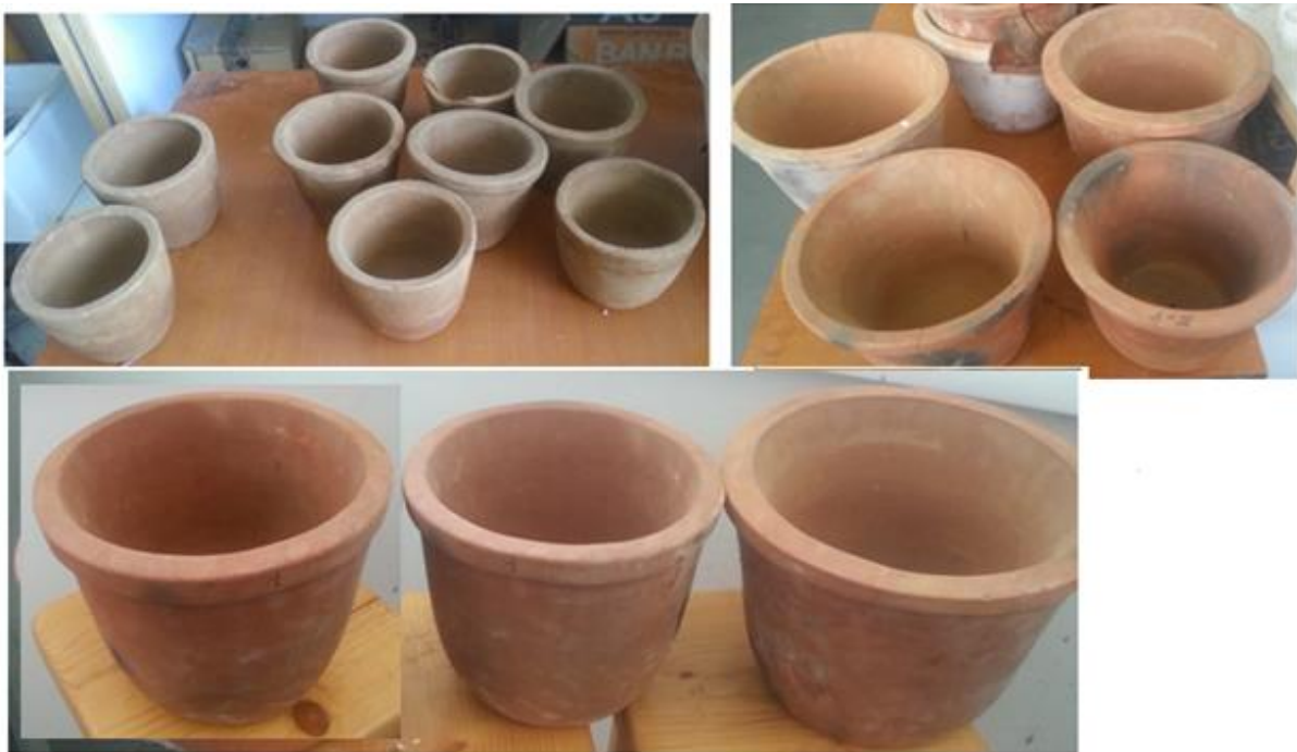
Figure 10. Some of the shaped and sintered filter elements produced.
