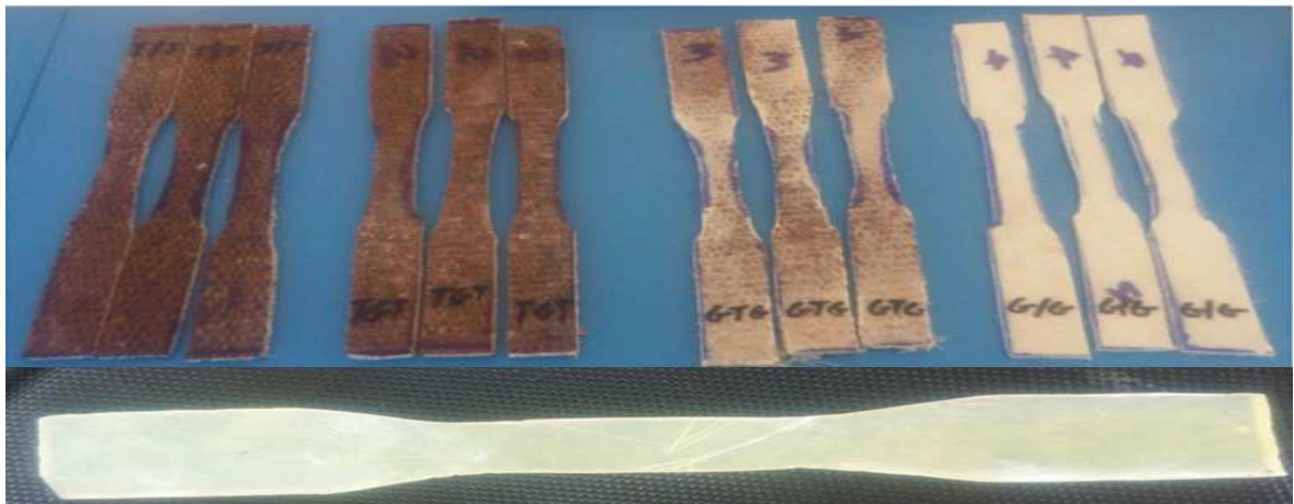
Figure 3.5. Tensile testing specimens
