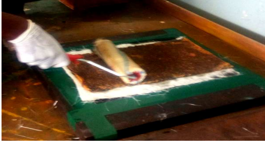
Figure 3.8. After cured the resin rolled for releasing bubble and for equal distributions of resin
