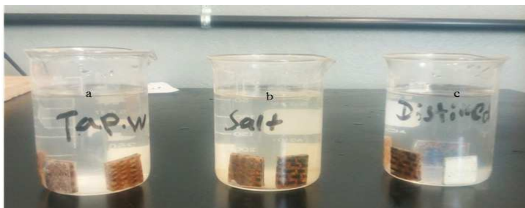
Figure 4.12. Water absorption test (a-tap water, b-salt solution water and c-distilled water)
