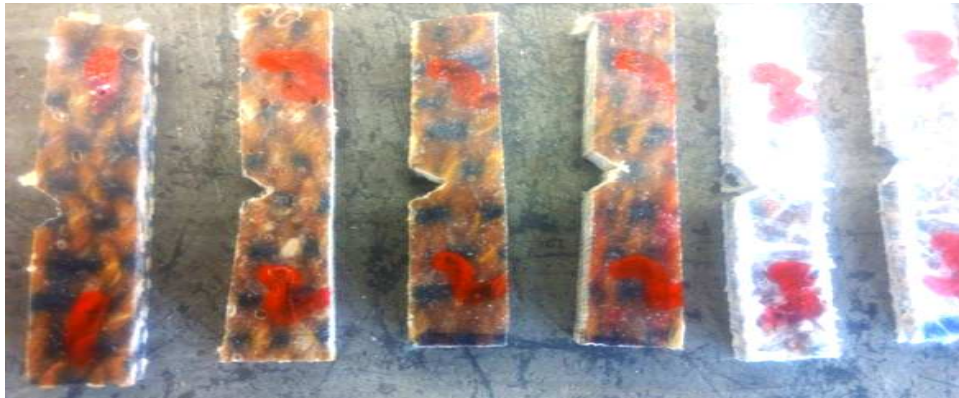
Figure 3.11. Impact specimens (ASTM-A370)
