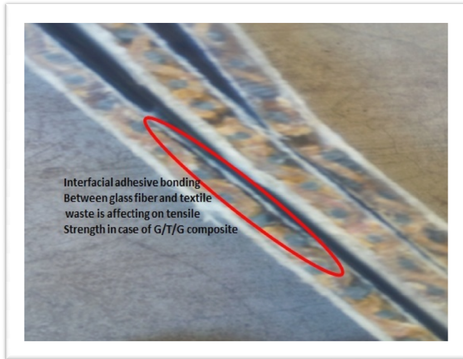
Figure 4.3. Rapture due to tensile load
