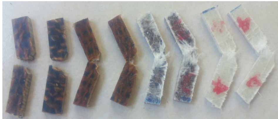
Figure 4.8. Ruptured specimens of hybrid composites due to impact load
