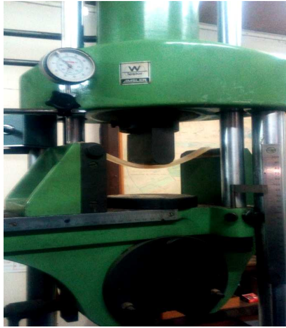
Figure 3.6. Universal bending test machine set up (Amsler product)
