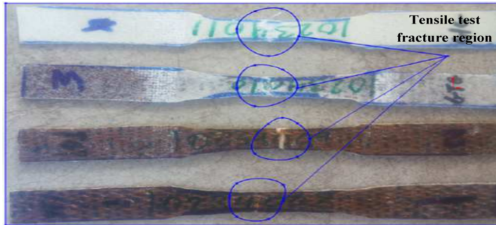
Figure 4.1. Ruptured specimens of hybrid composites due to tensile test load
