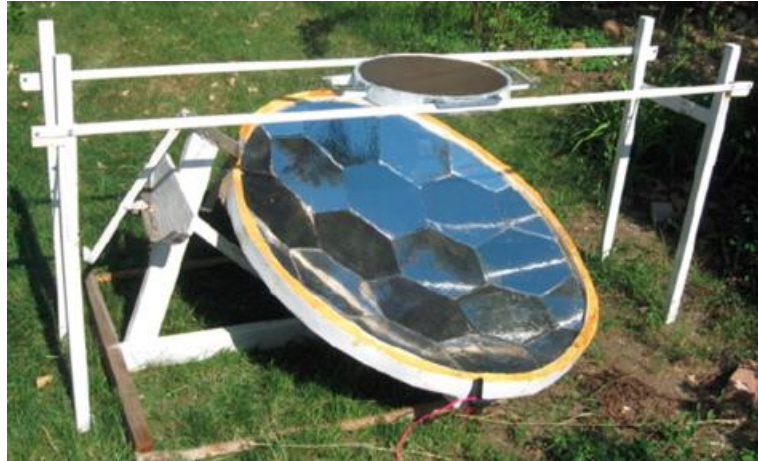
Figure 2.4: Concentric solar injera baking(Adem & Ambie, 2017)
