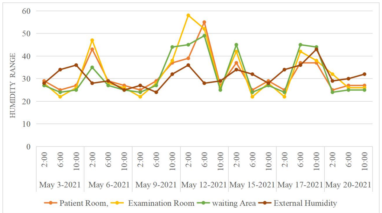
Figure 32. Humidity data of three indoor space and out door environment in May 2021 (field survey,2021)
