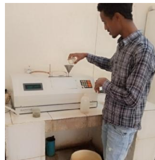
Figure 3.5 analysis of pol by polarimeter
