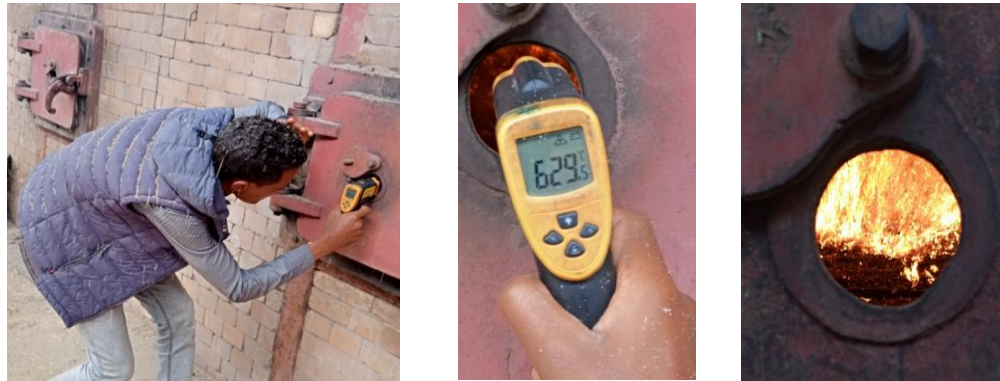
Figure 3.6 inside temperature of boiler furnace
