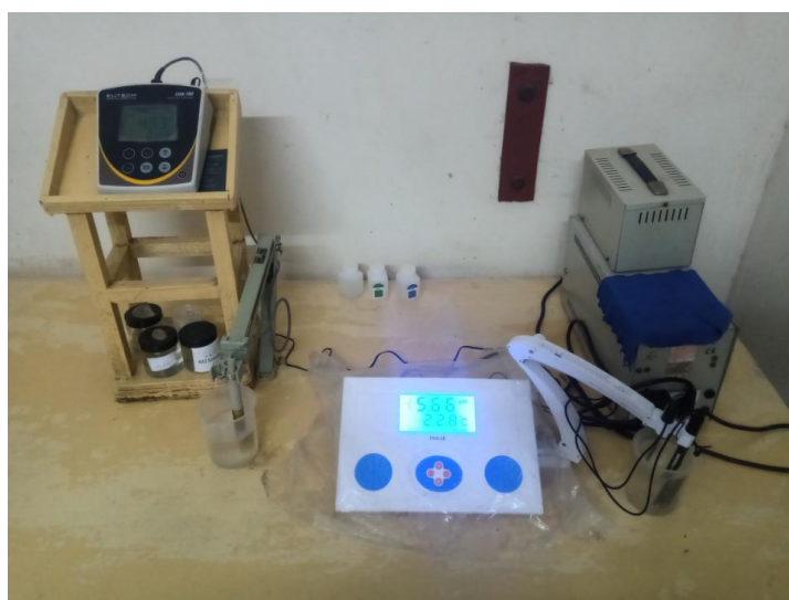
PH and Conductivity meter lab room of WSSF
