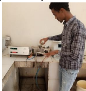
Figure 3.2 C.J & Syrup brix analysis by ABBE refractometer
