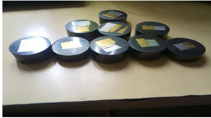
Figure 3.21: Prepared samples for microstructure and hardness test
