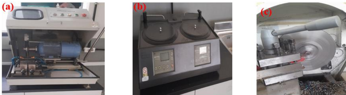
Figure 3.3: Specimen preparation (a) abrasive cutting (b) grinding and (c) Lath turning
