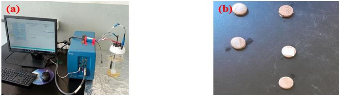
Figure 3.8: Corrosion resistance test setup (a) Instrumental setup (b) Prepared ample
