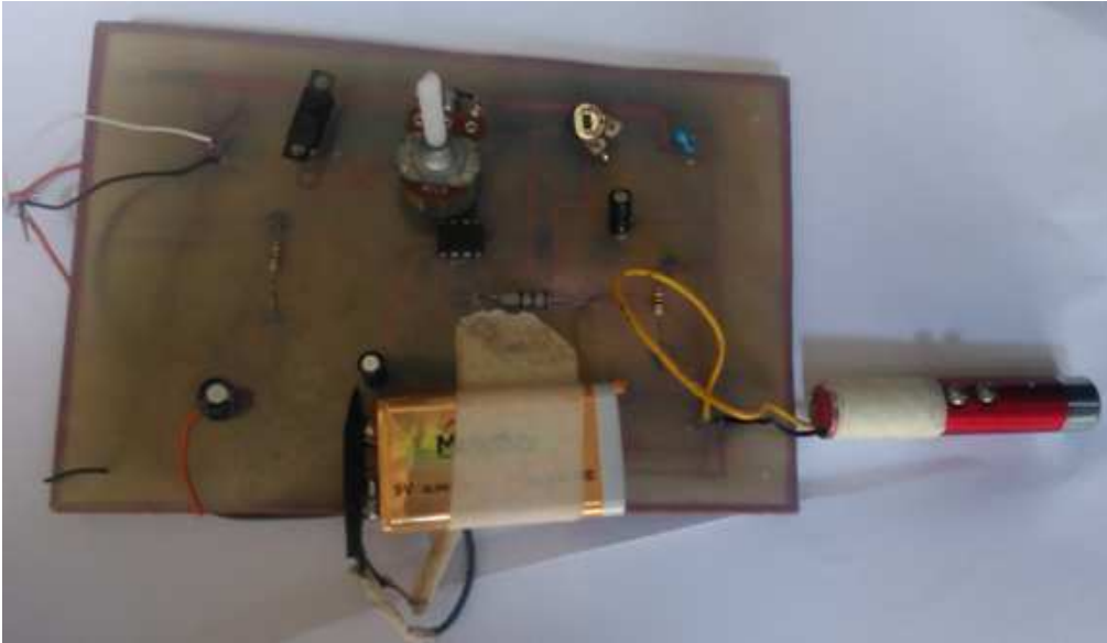
Figure 5.8: Transmitter of optical communication system for voice transmission.
