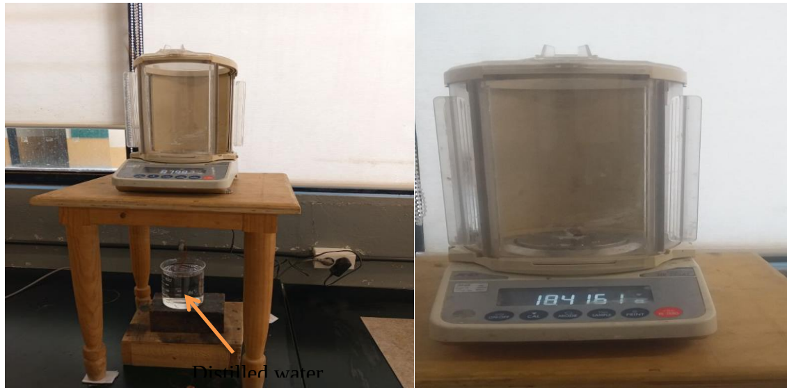
Figure 4.7 Measurement of density (a) measured in water (b) measured in air
