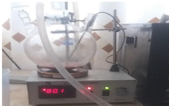
Figure 3.4 Dealumination of metakaolin using three necked round bottom flask setup.
