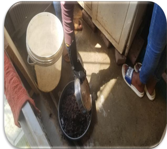
Figure 4.2 wet sieving of cinder material
