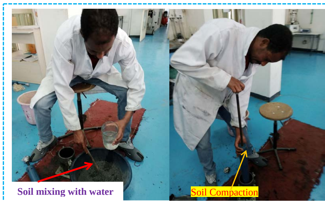
Figure 4.5 shows the soil laboratory compaction test
