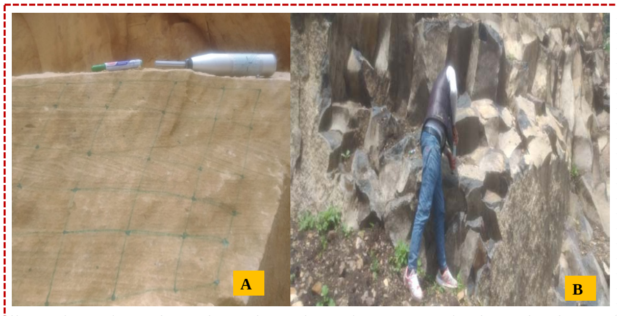
Figure 4.1 In-situ strength of intact rock using Schmidt hammer rebound test for the estimation of uniaxial compressive strength (UCS): A) preparing an equally spaced square of 25mm box and B) conducting the test with Schmidt hammer.
