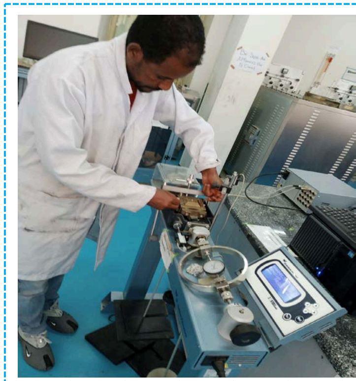
Figure 4.6 showing a direct shear test of soil in the laboratory.
