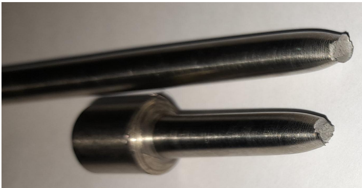
Tensile testing of 12.5 mm CP-Titanium grade 2 after failure
