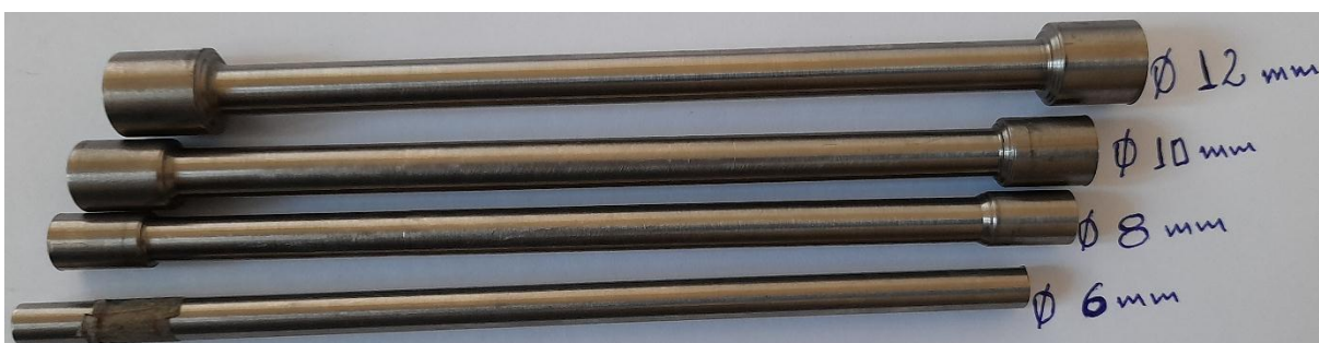
Prepared specimens of CP-titanium grade 2 rods for tensile test according to ASTM B348/ B348M-19.
