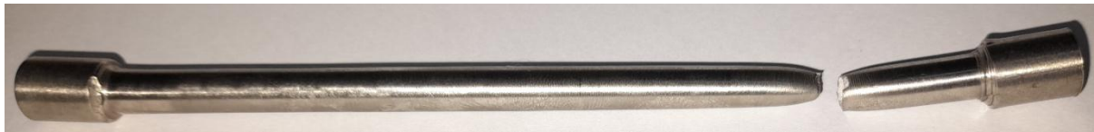
Tensile testing of 8 mm CP-Titanium grade 2 after failure
