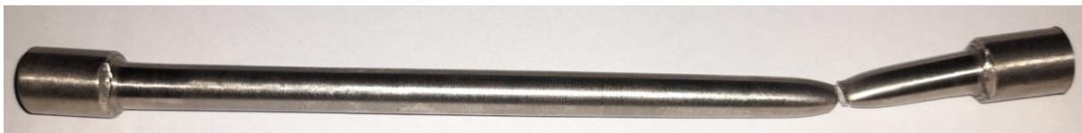
Tensile testing of 6 mm CP-Titanium grade 2 after failure
