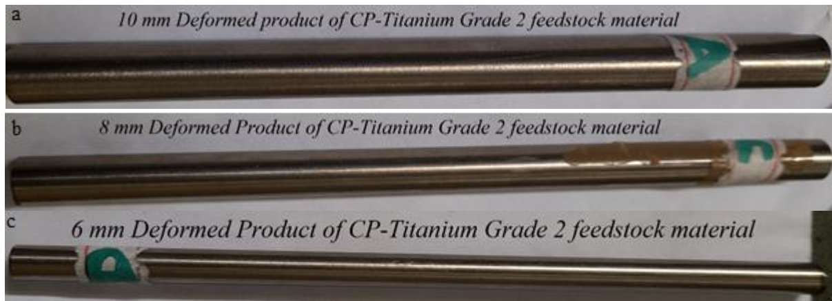
Figure 4. 51 Extruded product of CP-Titanium grade 2 feedstock material at a diameter of; (a) 10 mm, (b) 8 mm, and (c) 6 mm.
