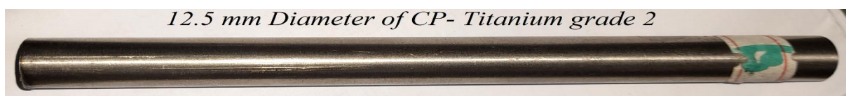
Figure 4. 50 CP-Titanium grade 2 feedstock material before deformation
