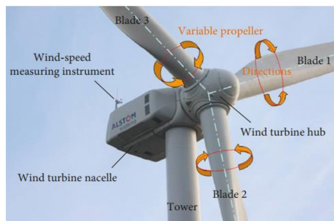
Figure 1.1 Blades action under pitch-controlled (Zhou & Liu, 2018)
