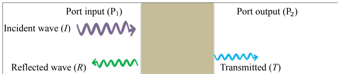
Figure 3: Showing port and scattering parameters. Port input (P 1 ) the left hand side, Port output (P 2 ) the right hand side. Incident wave (I) reflected wave (R), and transmitted wave (T)
