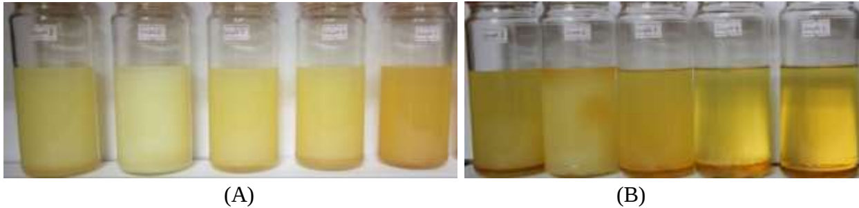
Figure 12. Sample fuels prepared for stability inspection, (A) before separation; (B) after separation
