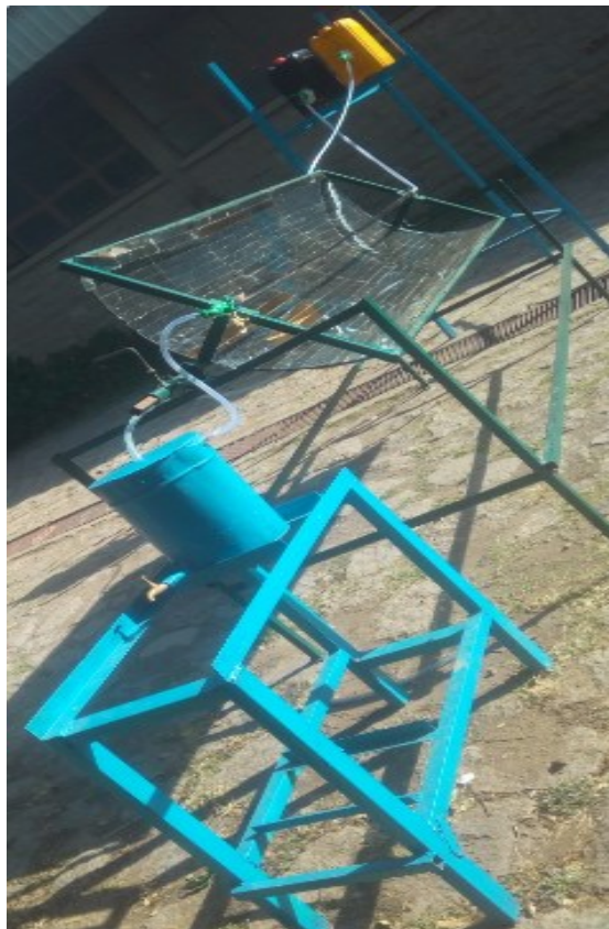
Figure 3.35 The schematic diagram for parabolic trough solar collector assembly for desalination.
