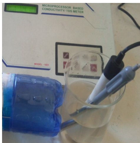
Figure 3.11 Conductivity before desalination
