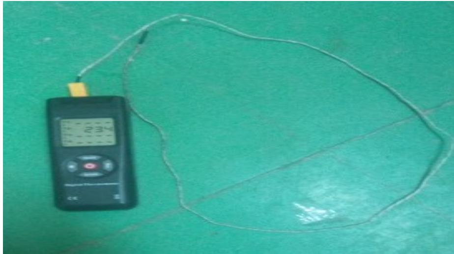
Figure 3.43 k type thermocouple ( digital thermometer)
