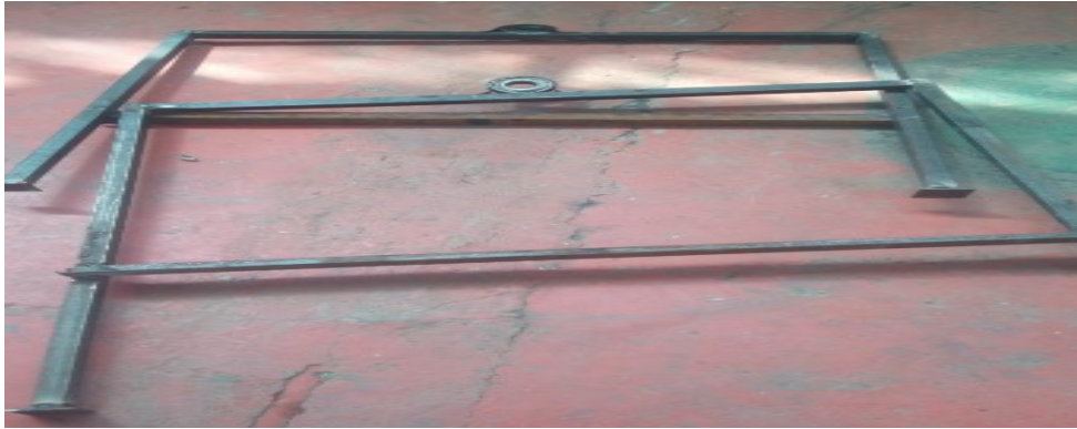
Figure 3.39 supporting stand for parabolic trough collector
