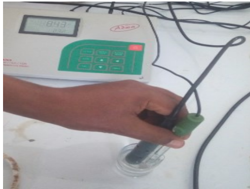
Figure 3.9 PH before desalination
