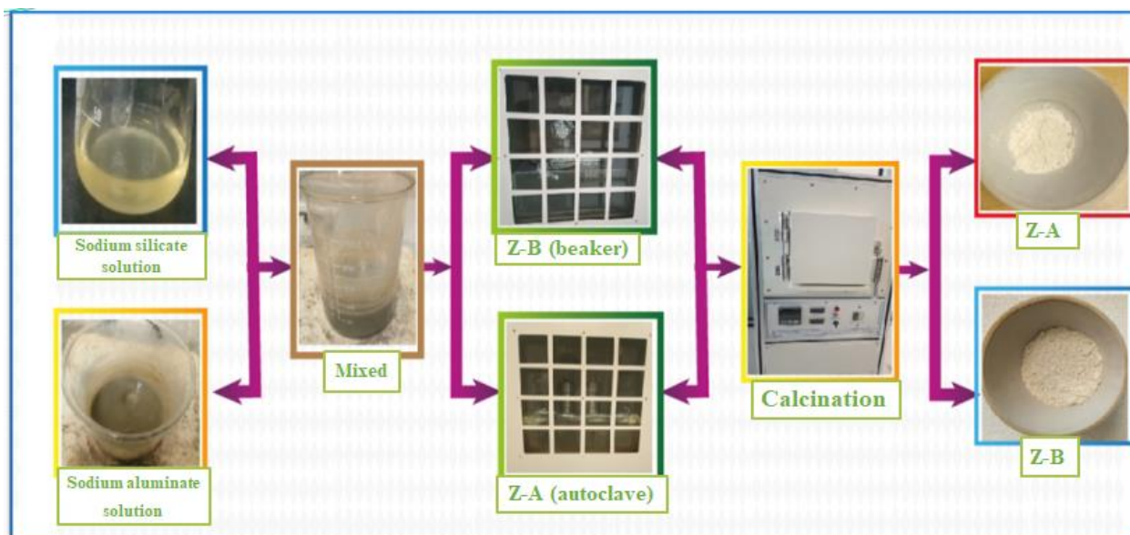
Figure 3.4: Schematics for the Synthesis of Zeolites by using different synthesis methods
