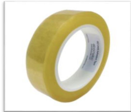
Tape for cross hatch cutter adhesiveness test
