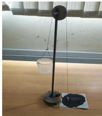
Fixed pulley system
