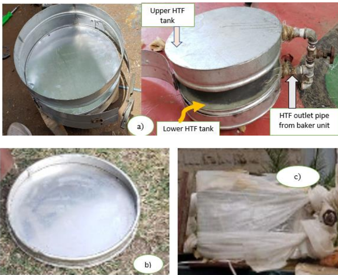
Figure 6. 6: - Manufacturing process of baker unit (a) baker unit with HTF tank (b) bread Patra (c) insulated baker unit
