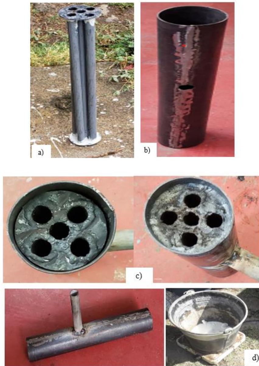
Figure 6. 5: - Manufacturing process of LHS (a) tube of LHS (b) shell of LHS (c) integrated of shell and tube and (d) PCM in container
