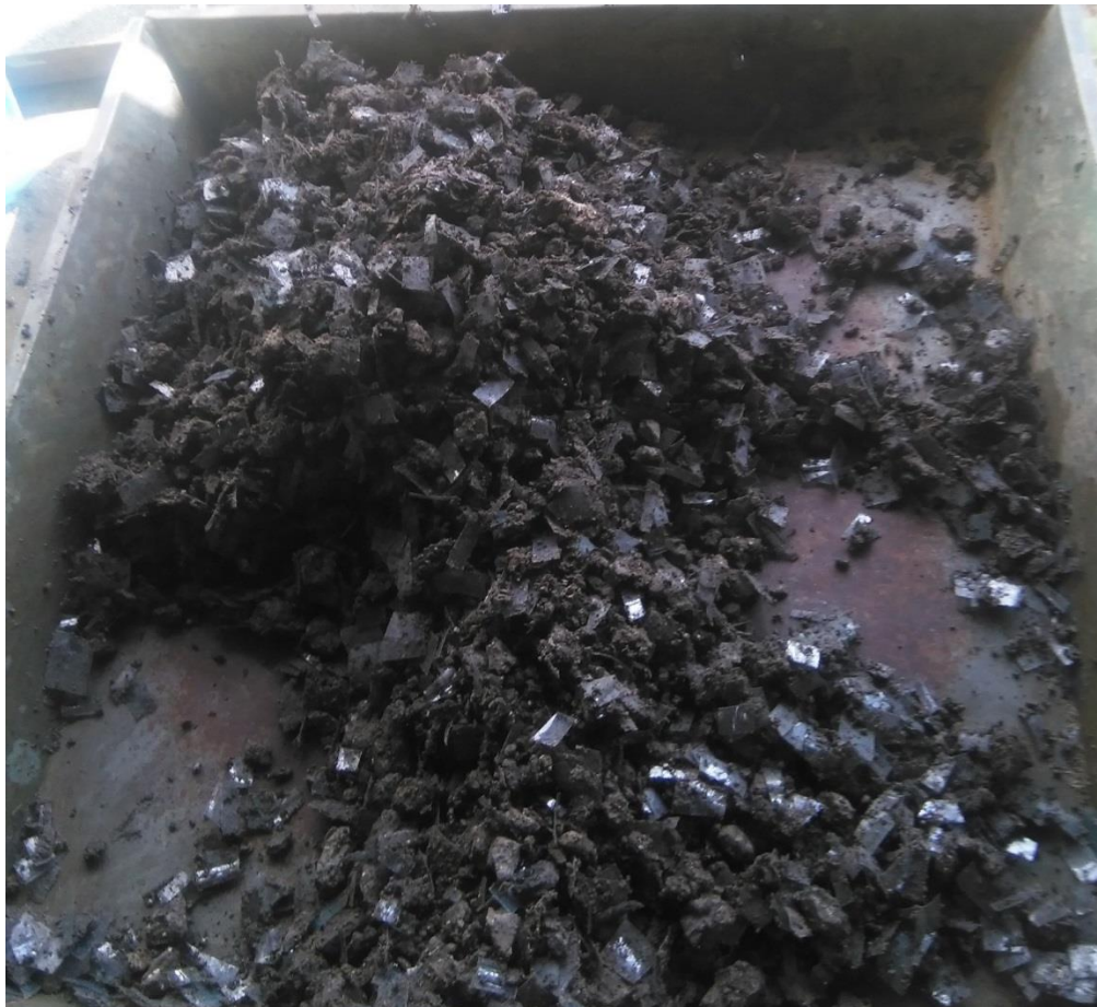
Figure.3.2 Soil mixing with plastic chips
