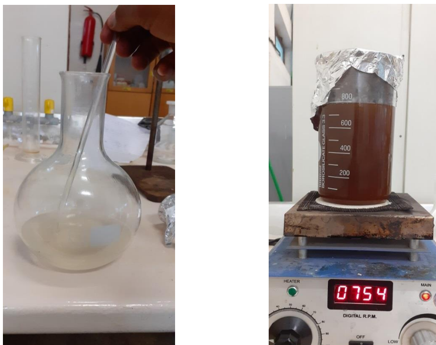
Figure 3.7 a) Dissolving NaOH in Methanol, b) Transesterification reaction on magnetic stirrer with hot plate
