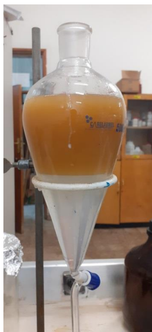
Figure 3.10 a) First round washed biodiesel, b) Final round washed biodiesel
