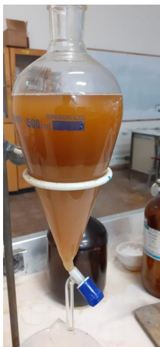
Figure 3.10 a) First round washed biodiesel, b) Final round washed biodiesel
