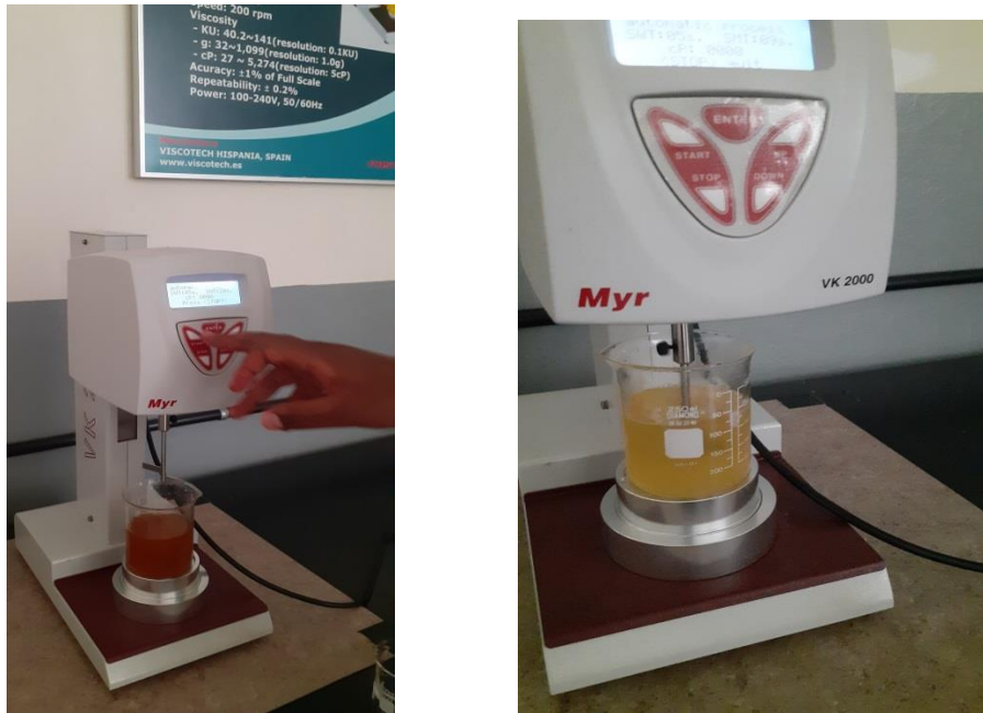
Figure 3.13 a) Measuring viscosity of biodiesel b) measuring viscosity of B20
