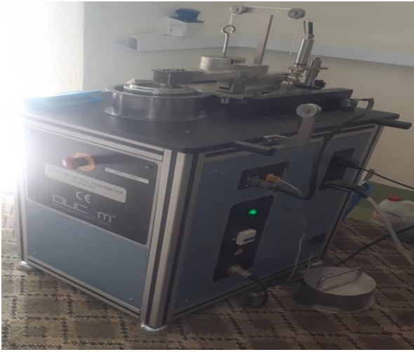
Figure 3.11 (A) Micro Pin on disk micrometer apparatus (B) wear rate analyzing software
