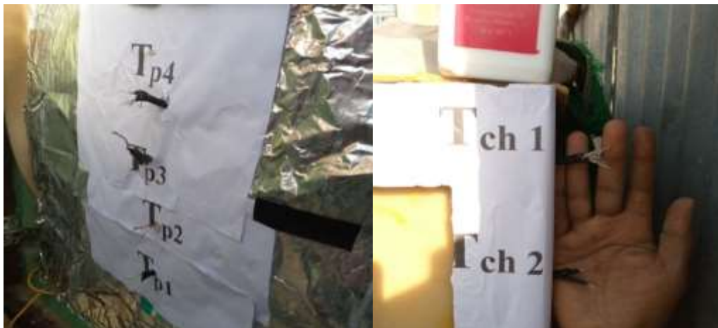
Figure 4.3 the thermocouple wires inserted into thermal energy material and for eggs chamber
