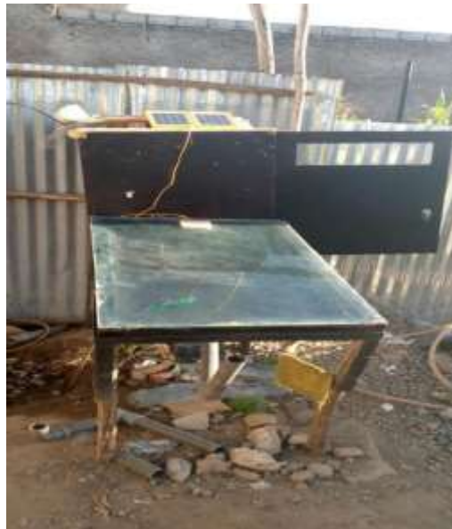
Figure 4.1 Solar Thermal Powered Incubator Systems
