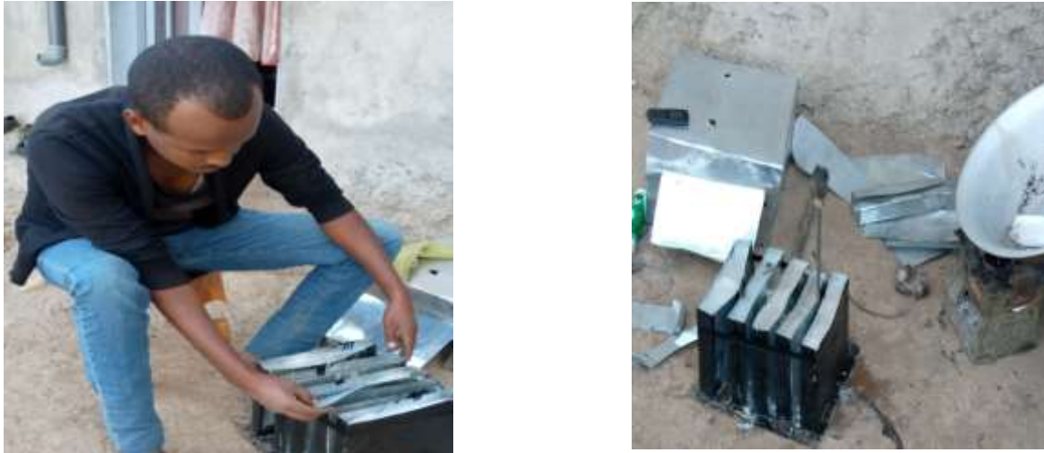
Figure 3.14 Preparing of thermal storage units
