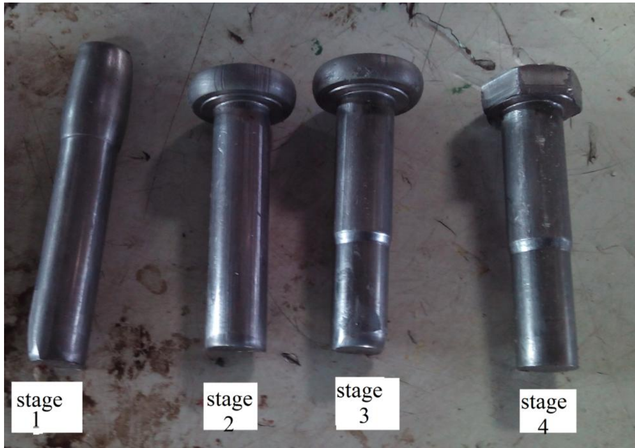
Figure 3.4 Bolt forming sequence
