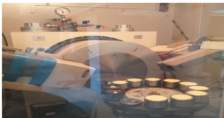
FIGURE 3.7: XRD testing setup of bamboo fibres
