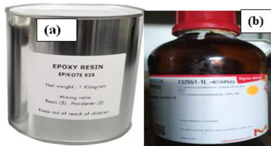
FIGURE 3.16: Resin for composite manufacturing (a) Epoxy 828, (b) hardener
