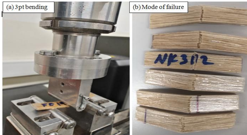
FIGURE 3.19: (a) Set-up for three-point bending test, (b) Mode of failure
