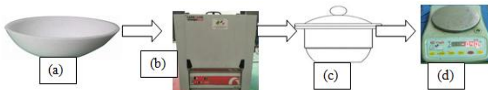
Figure setup of ash measurement (a) powder, (b) muffle furnace, (c) desiccators, (d) Oven
