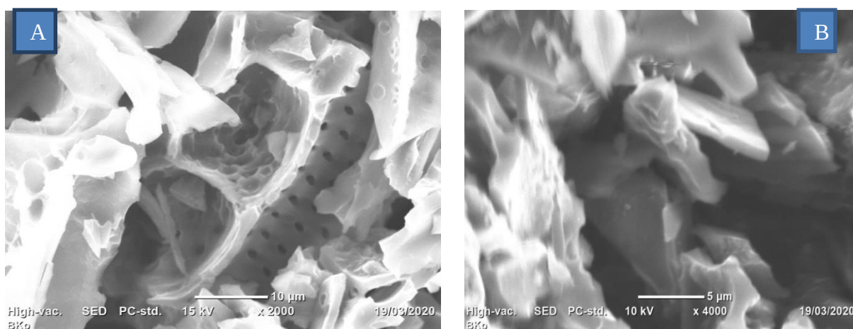
Figure3:SEM analysis of ACDKS before (A) and after (B) adsorption of Cr (VI) ions
