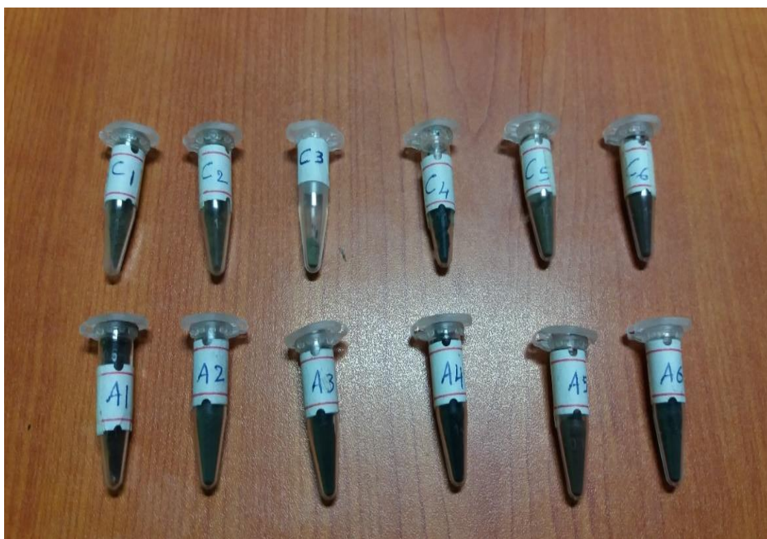
Figure 5. The six Ag NPs (A1, A2, A3, A4, A5 and A6) and six Cu/CuO NPs (C1, C2, C3, C4, C5 and C6) synthesised using the six medicinal plants.
