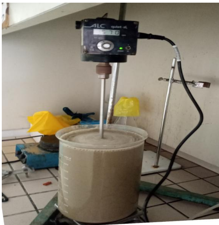
Figure 5b. Activation of purified bentonite with \text{Na}_2\text{CO}_3 and mechanical stirring
