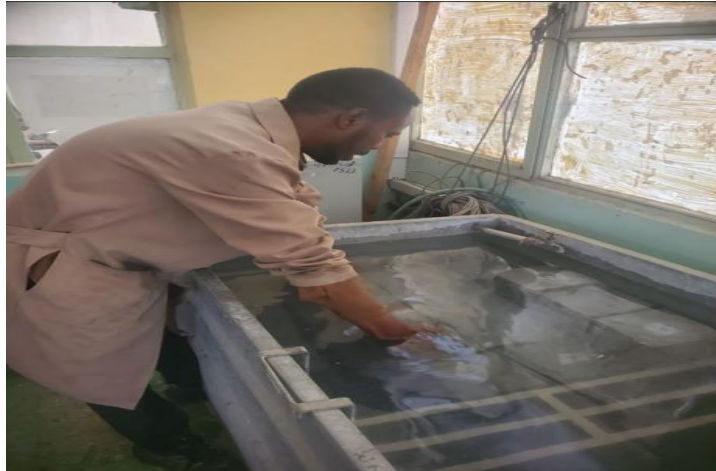
Figure 3. 4 Curing cube and flexural beam
