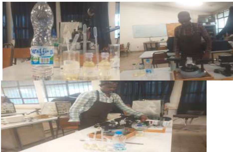
Figure 3.1 The samples Edible Oils and set up of prism spectrometer.
