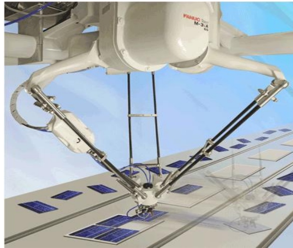
Figure 1. 2: A Delta Robot (Fanuc Delta Robot)( FANUC Robotics FOOD M-3iA/6S 4-Axis Remote A-Cab R-30Ib - Flexible Automation Supply, n.d. )
