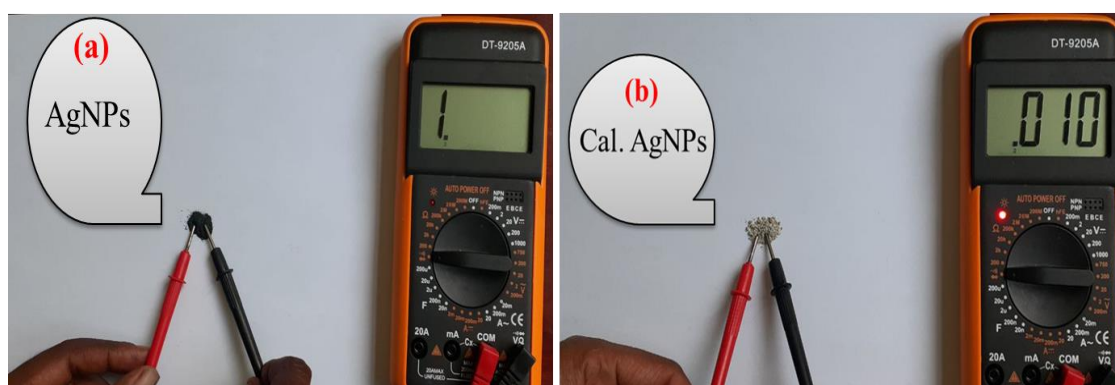
Figure 4-34: Continuity test of (a) AgNPs without calcination (b) Calcined AgNPs by digital multi-meter
