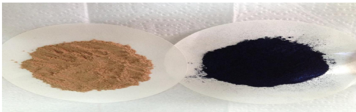
Figure 3. 2 Palm seeds before and after MB adsorption.
