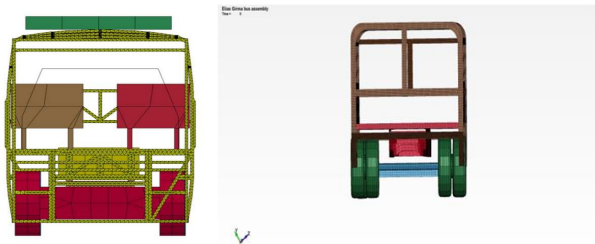
a) Full-scale rollover test arrangement b) FE analysis rollover test arrangement
