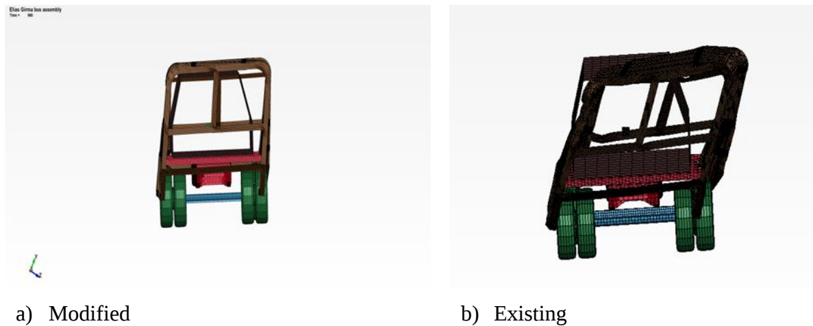
Figure 5.26. Structural response a) modified and b) existing Isuzu bus
