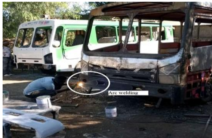
Figure 4.16. Isuzu bus joining process
