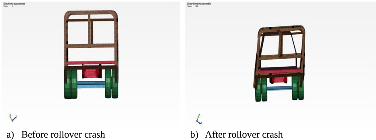
Figure 5.19. Modified Isuzu bus a) before and, b) after rollover crash
