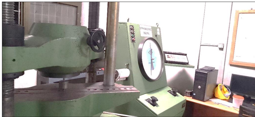
Figure 3.11 The Universal Testing Machine (UTM) for compression test
