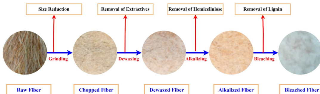
Figure 27. Flow chart of extraction process for non-cellulosic components removal
