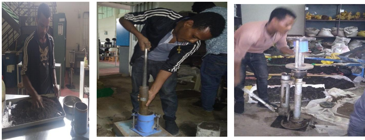
Figure3.4 Standard compaction tests
