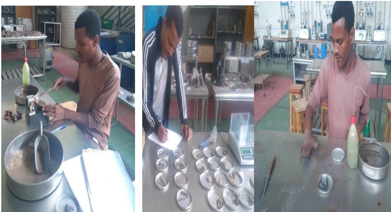
Figure3.3 Atterberg limit tests
