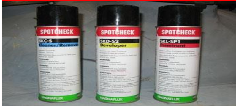
Figure 3.4 Dye Penetration Test (MIDI lab)
