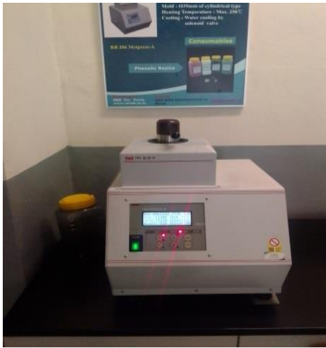
Figure 3.6 Mounting machine (ASTU)
