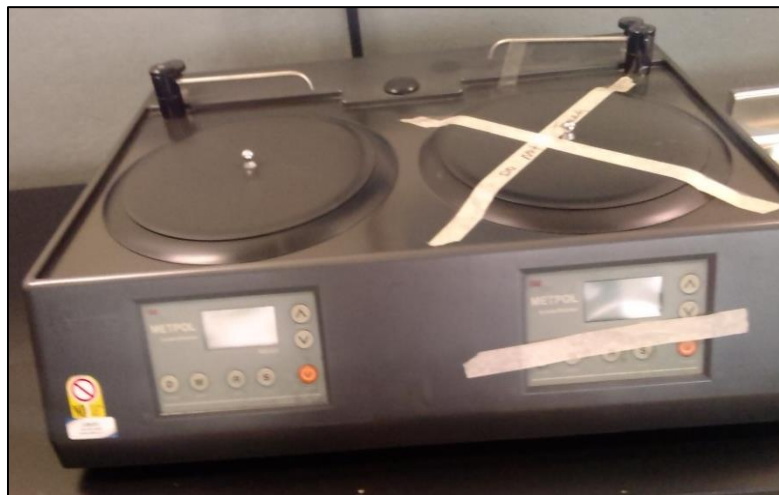
Figure 3.8 Grinder/polisher (ASTU material lab)
