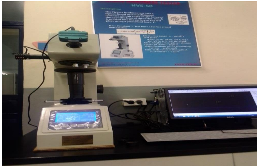
Figure 3.9 Vickers hardness testing machine (ASTU material lab)
