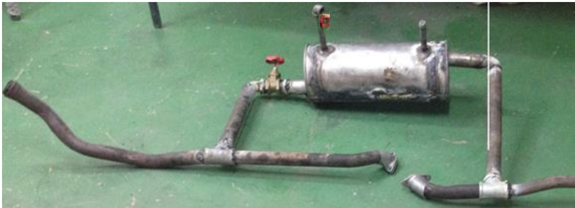
Figure 3.6: Manufactured EGR cooler system assembly for the conventional engine modification
