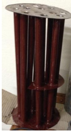
Figure 3.5: Assembly of cooler tubes and baffle plates
