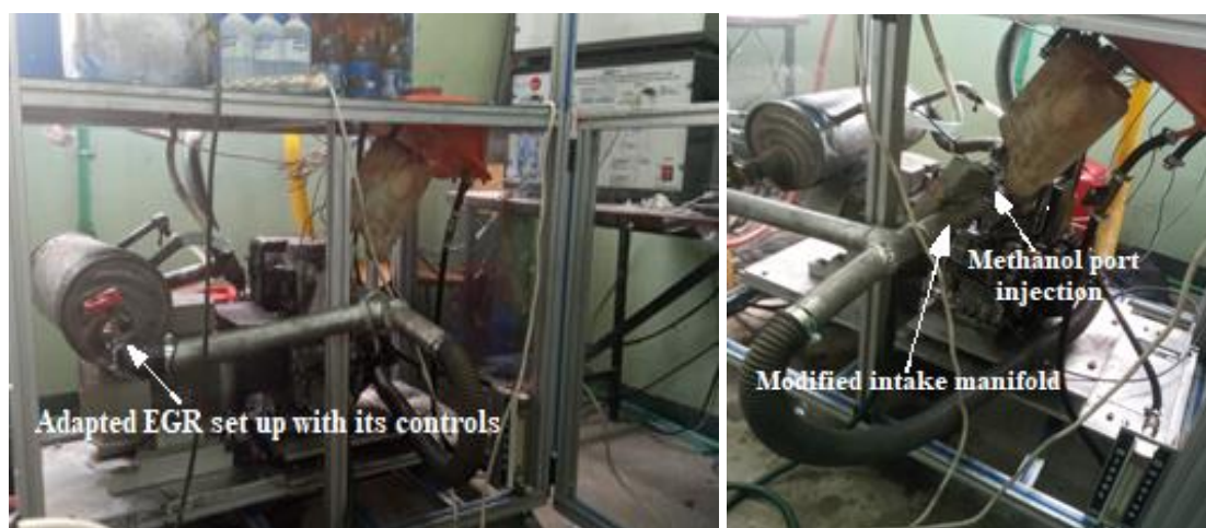
Figure 3.8 Modified intake manifold and adapted EGR set up
