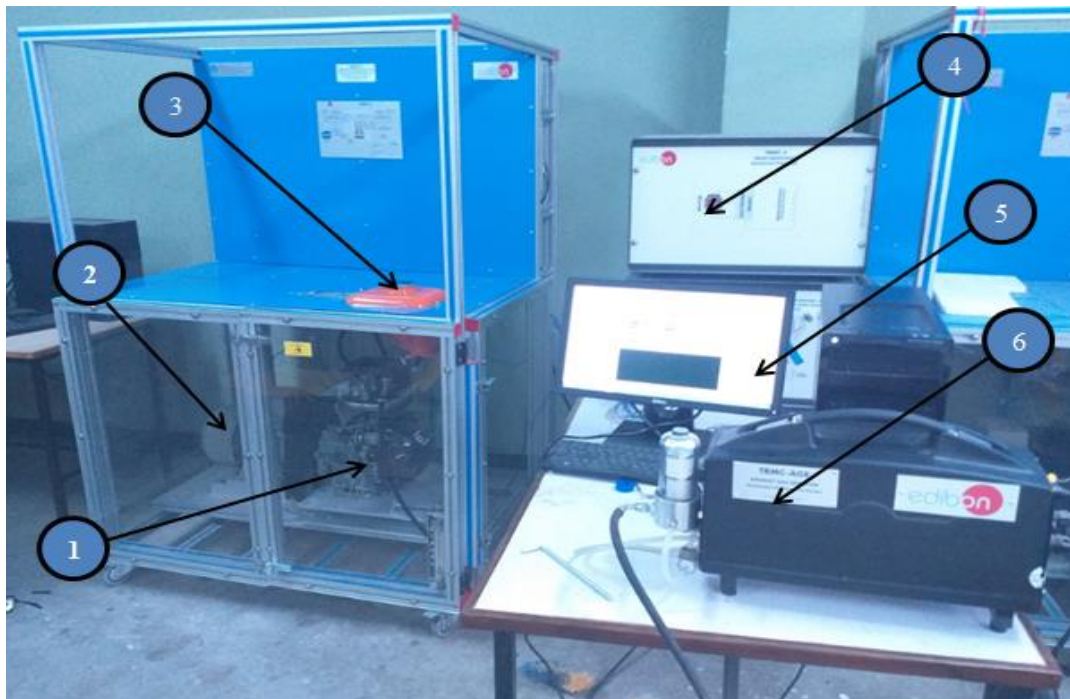
Figure 3. 7: Experimental setup of TBM3-02 test bench for single-cylinder diesel engine
