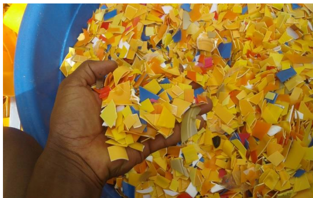
Figure 3. 2: Shredded waste plastic for pyrolysis.
