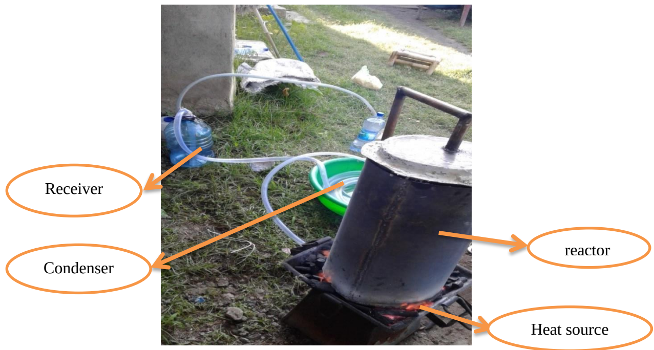
Figure 3. 1: Simple batch reactor for waste plastic pyrolysis.
