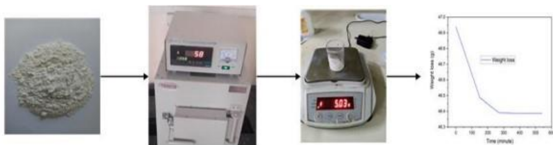
Ash content determination of native cassava starch
